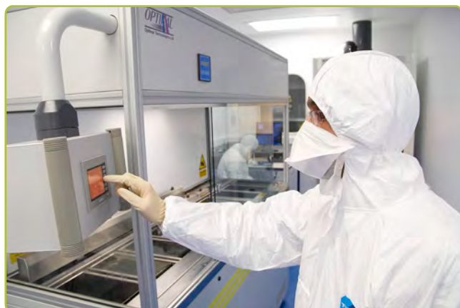
Left: Microfluidic devices are fabricated in Dolomite's class-1000 cleanroom
