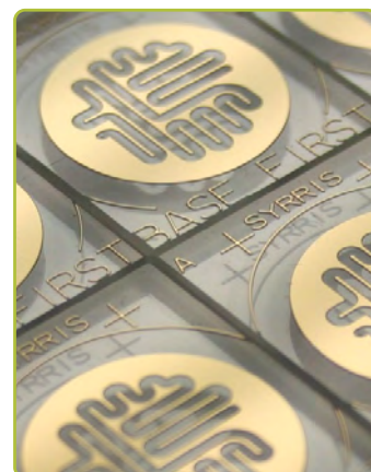
Left: Microfluidic devices are fabricated in Dolomite's class-1000 cleanroom
